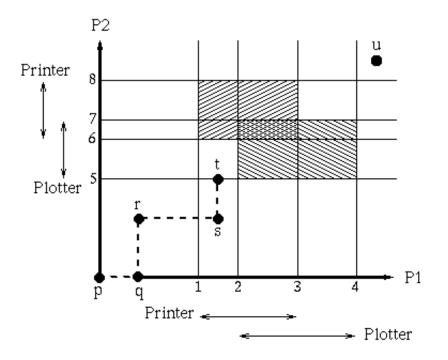
The horizontal and vertical axes represent the number of instructions executed by P1 and P2 respectively. The dashed line is a *resource trajectory*; it shows when the scheduler ran each process P1 and P2. Suppose that  $\mathbf{p}$  is the initial situation and the  $\mathbf{u}$  is the final point. Process P1 must pass lines 1, 2, 3, and 4 and process P2 must pass lines 5, 6, 7, and 8.
